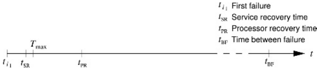
Fig. 4. The relation between the service and processor recovery periods and the time between failures
